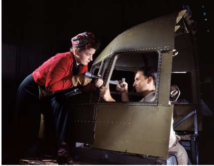
Inglewood, California. Riveting team working on the cockpit shell of a C-47 heavy transport at North American Aviation
